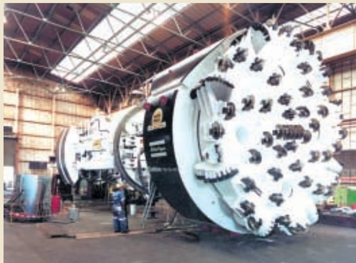
Tunnel boring machines (TBMs) will be used in the construction of the twin rock tunnels.
