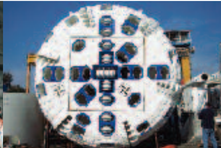
Tunnel boring machine
