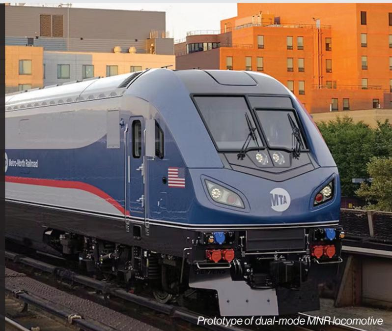
Prototype of dual-mode MNR locomotive
