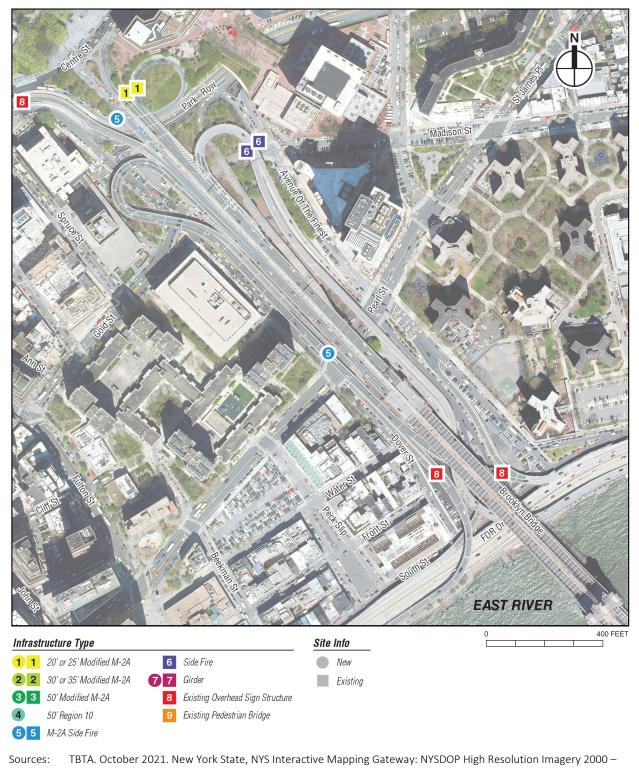
Figure 2-2f. Proposed Locations of Tolling Infrastructure and Tolling System Equipment: Brooklyn Bridge
