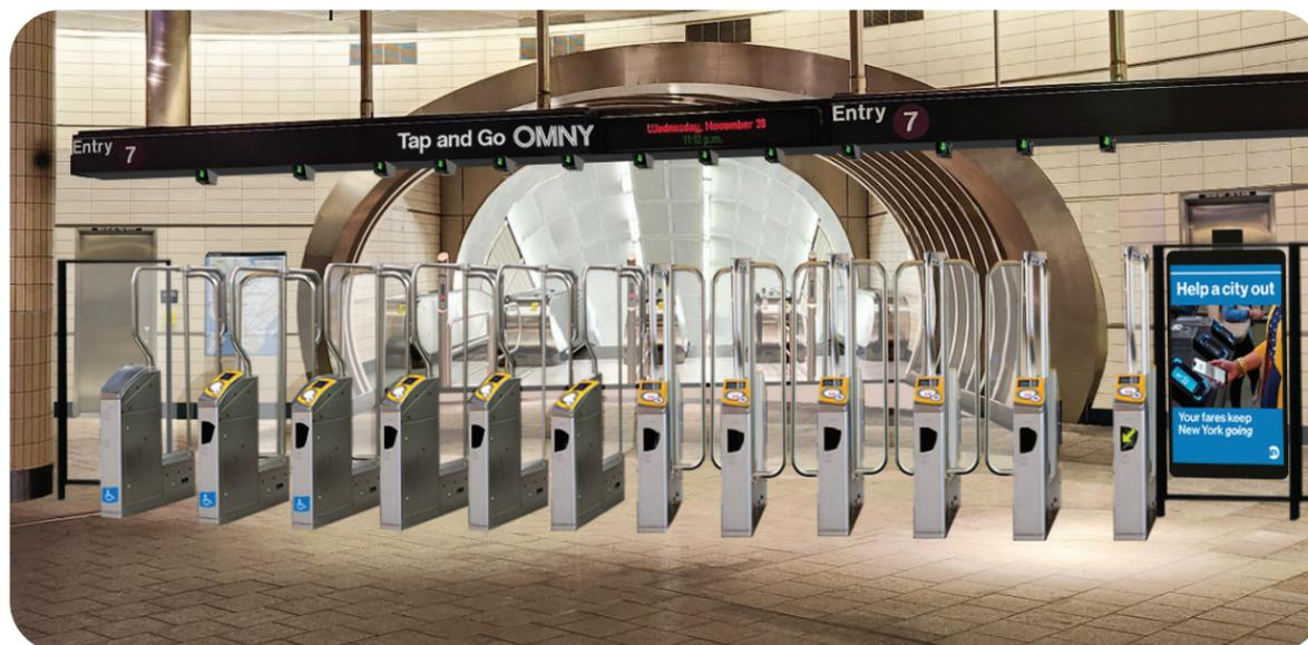
Figure 20 Rendering: Hudson Yards with potential "faregates of the future," including motorized swinging plexiglass entry/exit doors in place of turnstiles; overhead array combining sensors (green lights), digital customer service and fare payment messaging; and clear plexiglass fencing where emergency exit gates are today.
