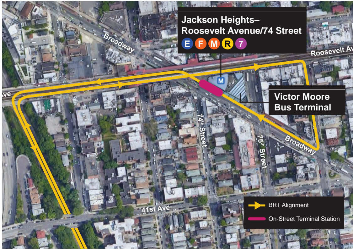
BRT alignment along Roosevelt Avenue and Broadway.
