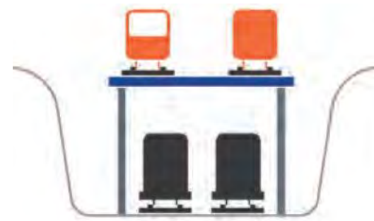
Figure 1: Typical profile views of BRT/LRT alignments in Brooklyn before and after revision Original Profile and Conceptual Cross Section
