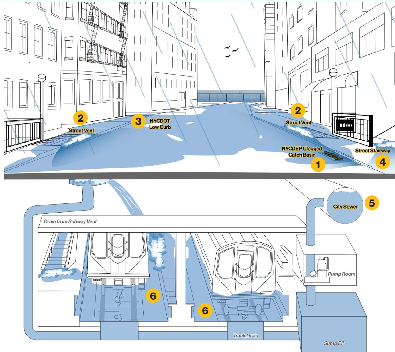
When large volumes of stormwater enter through vents and down street stairs, and when **city sewers (5)** are full and backup into stations, the underground drainage system becomes taxed. Stormwater can build up in mezzanines and on stairways and platforms, impacting customer experience. Subway service delays occur when **stormwater floods tunnels and tracks (6)**. Subway service is shut down until the water is removed.
