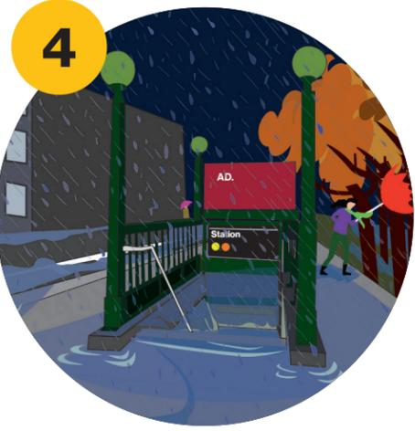
**Low curb heights** near subway entrances can't hold back stormwater from flowing over streets and sidewalks and down subway street stairways, to the mezzanine.
