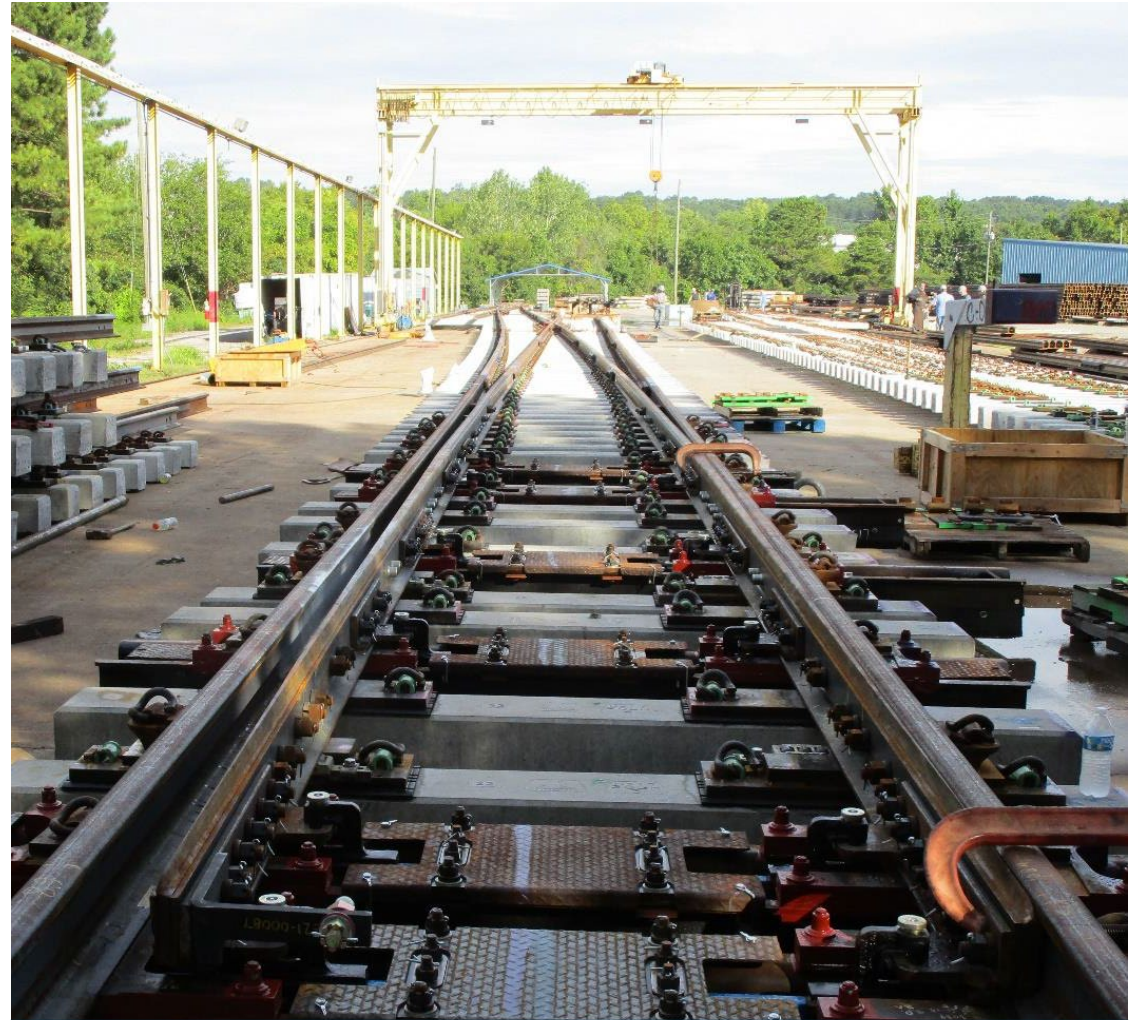
Factory test of fabricated railroad crossovers and switches at Voestalpine Railway Systems Nortrak facility in Birmingham, Alabama, August 2022
