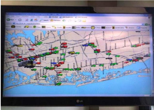
**Figure 14: Real-time GPS tracking of support vehicles and snow-fighting equipment aided decision-makers in the LIRR situation room**
