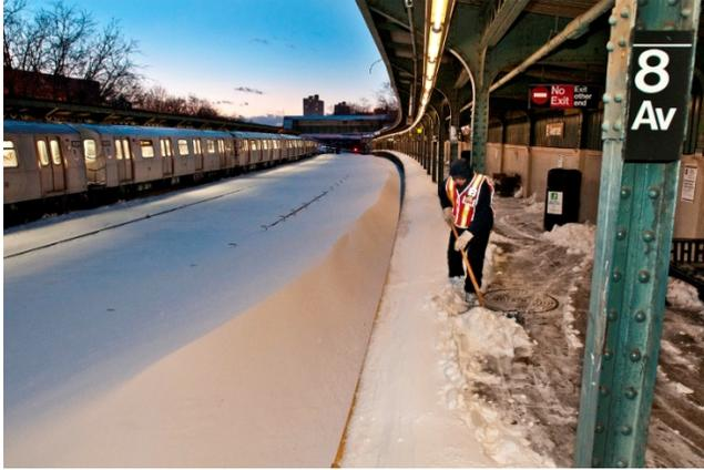
**Figure 6: Open cut subway lines were vulnerable to snow accumulation and required several days to be cleared**
