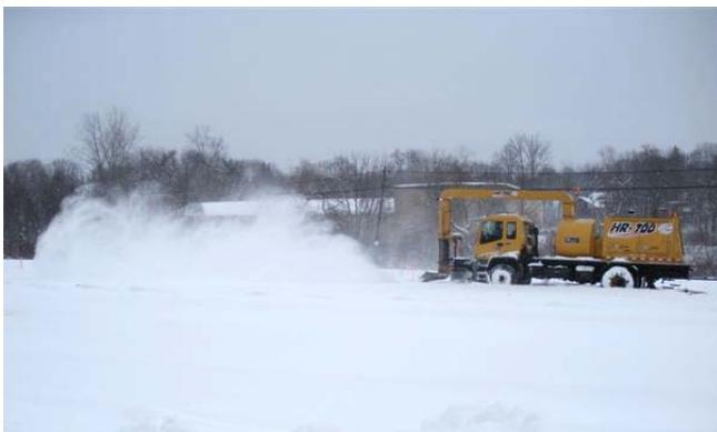
**Figure 15: Cold air blowers such as this one at Metro-North can rapidly clear snow**
