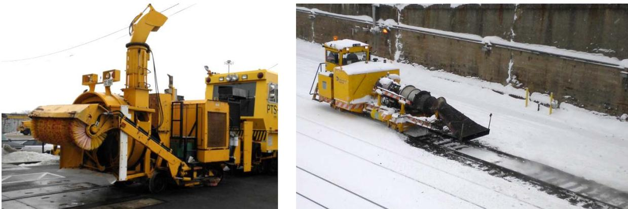
**Figure 5: Specialized snow-fighting equipment complemented manual labor in clearing snow (LIRR snow broom at left, Metro-North jet blower at right)**
