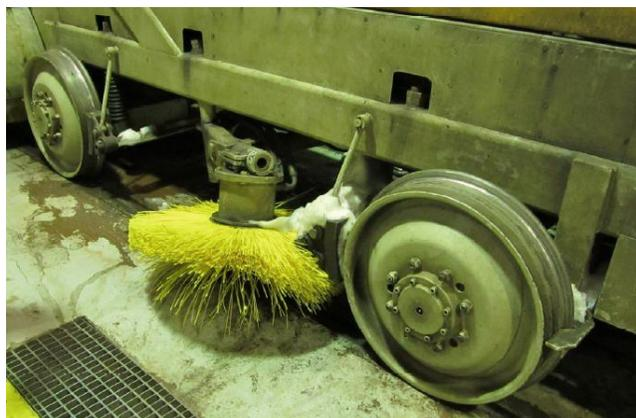
**Figure 16: This novel machine from Finland can help to clear third rail snow and ice buildup**
