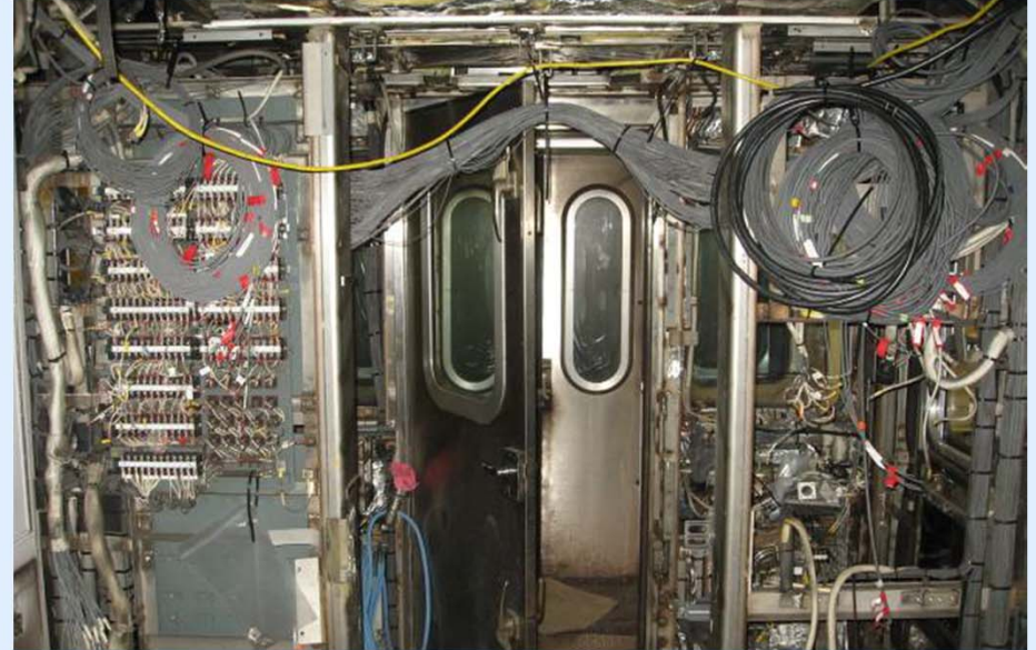
#7265 Cab Wiring - Conversion Work
