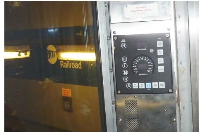
Installed Cab Car PTC ADU
