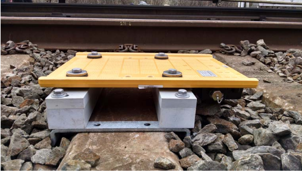
Transponder on Concrete Tie
