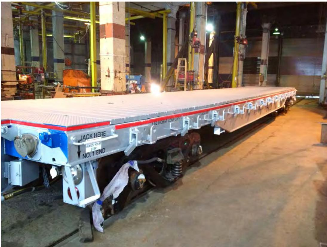
Flatcars are used to transport equipment and materials to work sites. Photos show before and after images of flatcar frame repair. These refurbished flatcars will support ongoing maintenance and construction activities.
