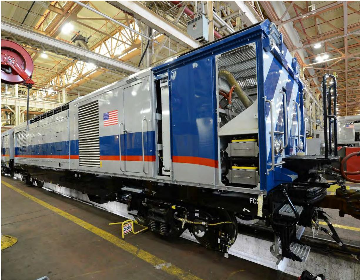
This is the first of three new vacuum trains purchased by NYCT. This train is currently undergoing acceptance testing and is expected to be put in service shortly. The vacuum trains are used to remove debris from the track which can cause fires and block drains.
