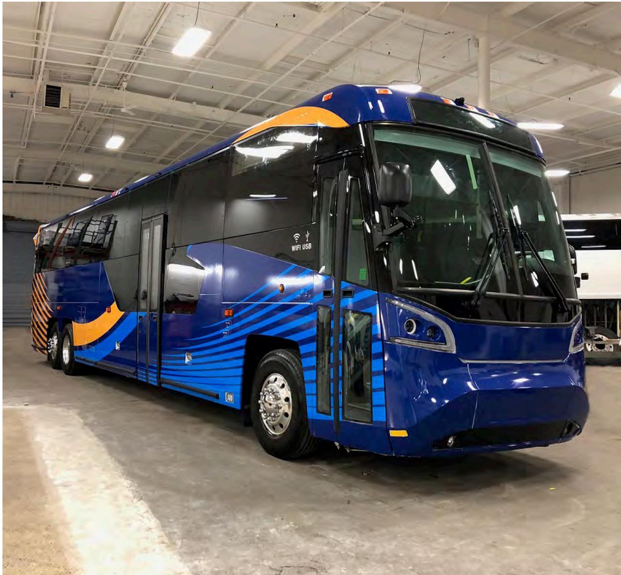
A newly reimagined commuter coach being prepared for a three month pilot at NYCT. This bus features an innovative low-entry vestibule with a ramp and adjoining seating area designed to improve accessibility, as well as Wi-Fi, and USB ports.
