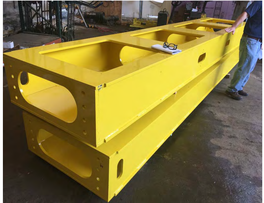
Drop Table Electrical Traversing Structures in Fabrication
