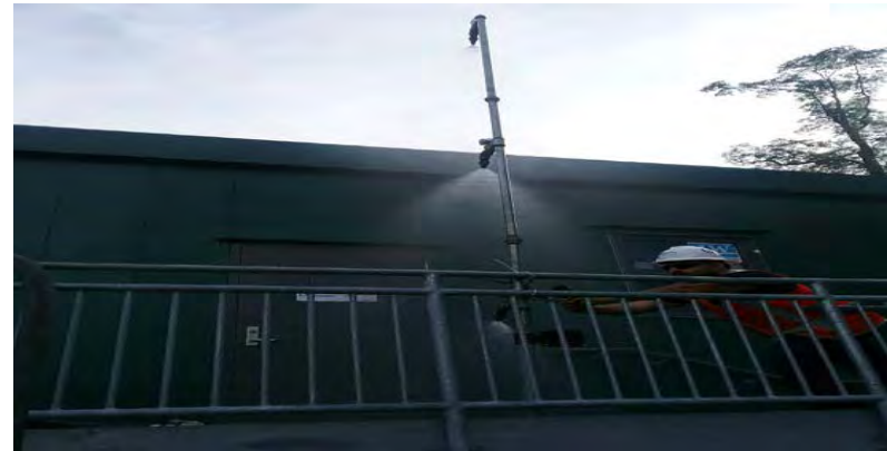
Water testing at Riverdale substation
