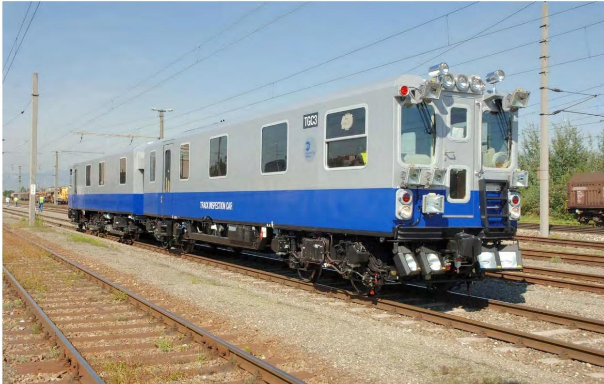
Pictured above is one four Track Geometry Cars, self-propelled diesel railcars capable of measuring rail, track and tunnel geometry under dynamic loading conditions. The cars have a series of onboard measuring and analyzing systems, as well as propulsion, braking and power generation units that enable them to perform their measuring and inspection tasks at allowable train speeds. These cars measure and confirm important components of track safety.
