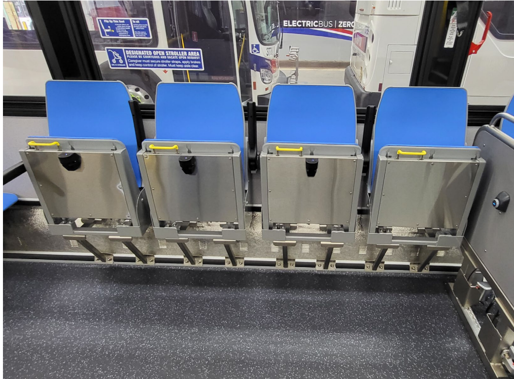
Continuous flip-up seats provide flexible seating for walkers, strollers, etc.
