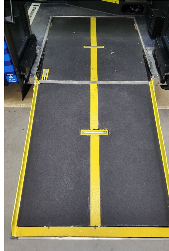
Wider 32-inch ramp with center line provides better accessibility for various mobility devices.
