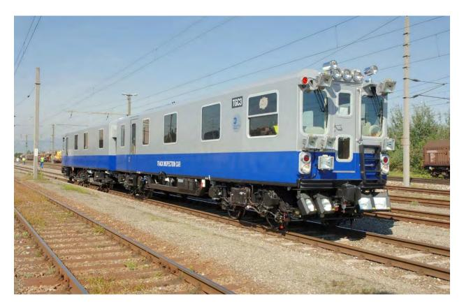
Pictured above is one four Track Geometry Cars, self-propelled diesel railcars capable of measuring rail, track and tunnel geometry under dynamic loading conditions. The cars have a series of onboard measuring and analyzing systems, as well as propulsion, braking and power generation units that enable them to perform their measuring and inspection tasks at allowable train speeds. These cars measure and confirm important components of track safety.
