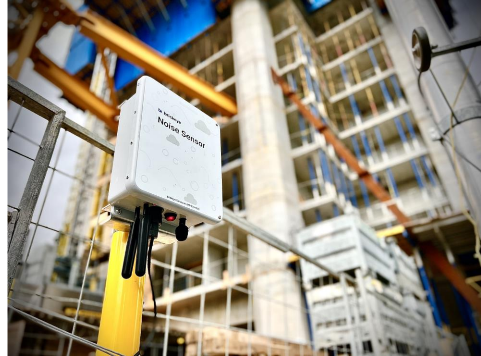
Noise Monitoring Device
