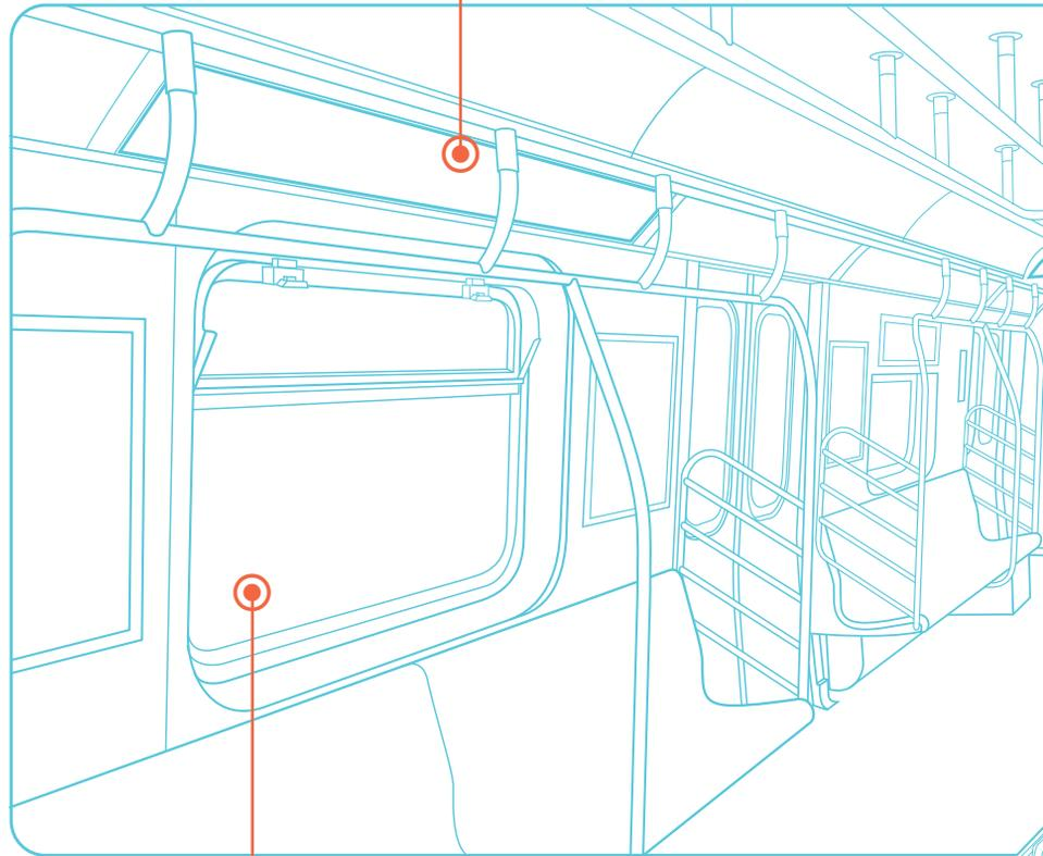
Protective layer of replaceable film on window glass prevents permanent scratching
