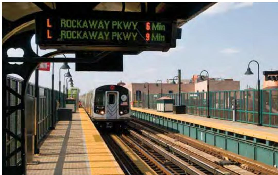
As we modernize some signals, we're replacing others with a new computer-based system that knows the precise location of every subway train on the tracks and can automatically space trains closer together. This system—which is fully in place on our subway's L Line—allows us to run more trains and provide better service.
