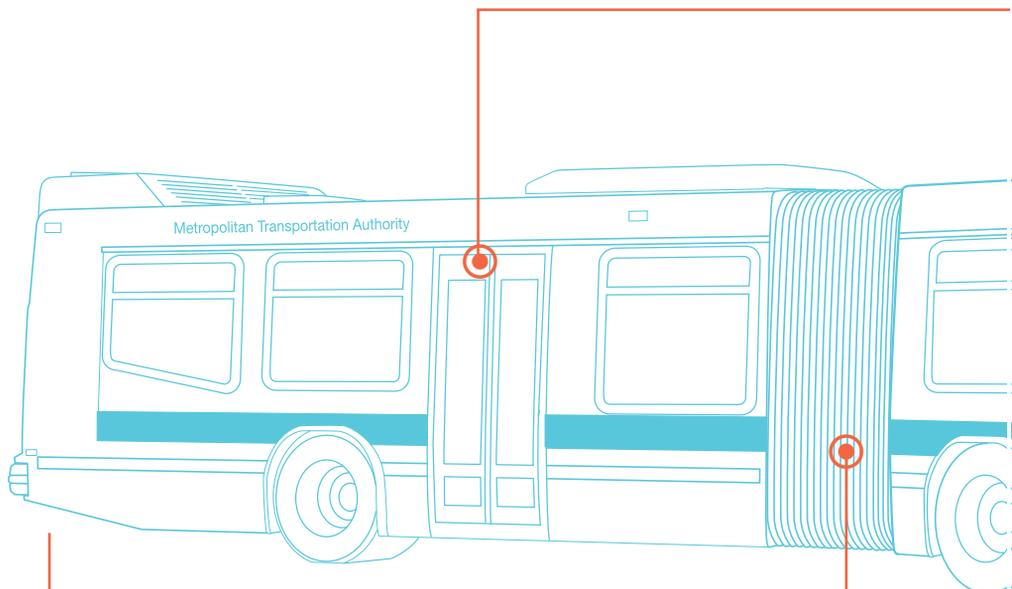
"Accordion" center bends in the middle, allowing high-capacity bus to turn within the same radius as a regular 40 foot bus
