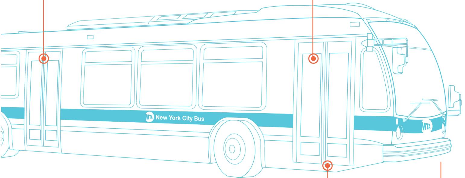
Low-floor design better supports heavy loads and allows faster boarding for wheelchairs and elderly passengers
