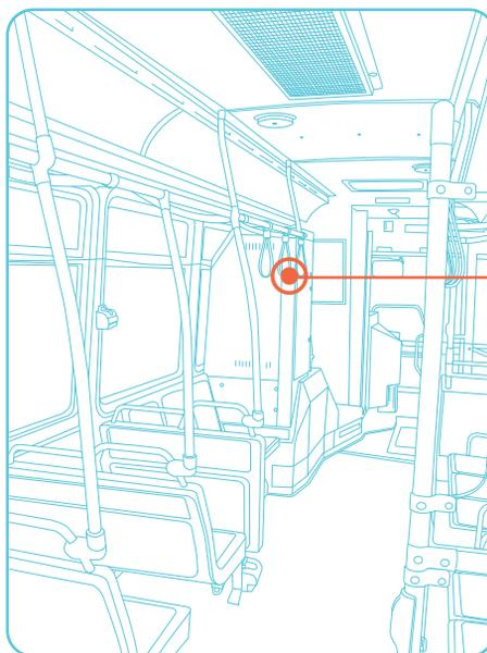
Electronic compartment houses special equipment for services like MTA BusTime, which gives customers real-time bus information via cellphone
