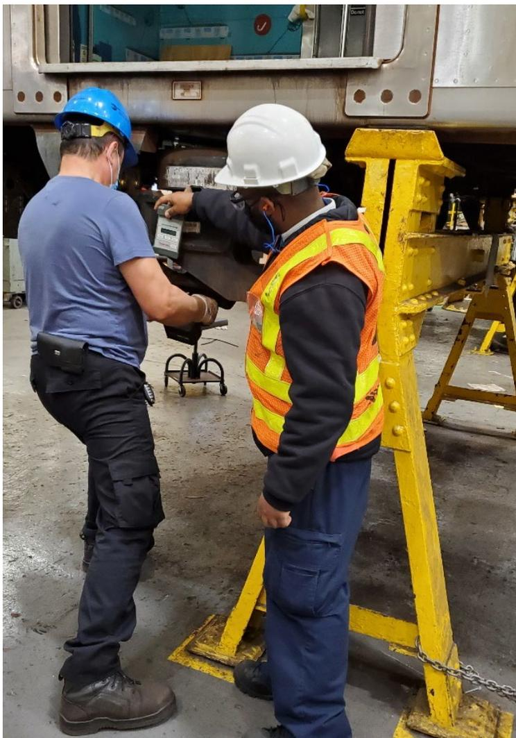
System Safety Specialist Sebastien Ruban at the Coney Island Overhaul Car Repair Shop during the installation and securing of bolsters. Screening measurements were taken with a direct read sampling device (DataRAM) to ascertain the airborne concentration of particulate matter to determine if the job task must be included in NYCT's Respiratory Protection Program.
