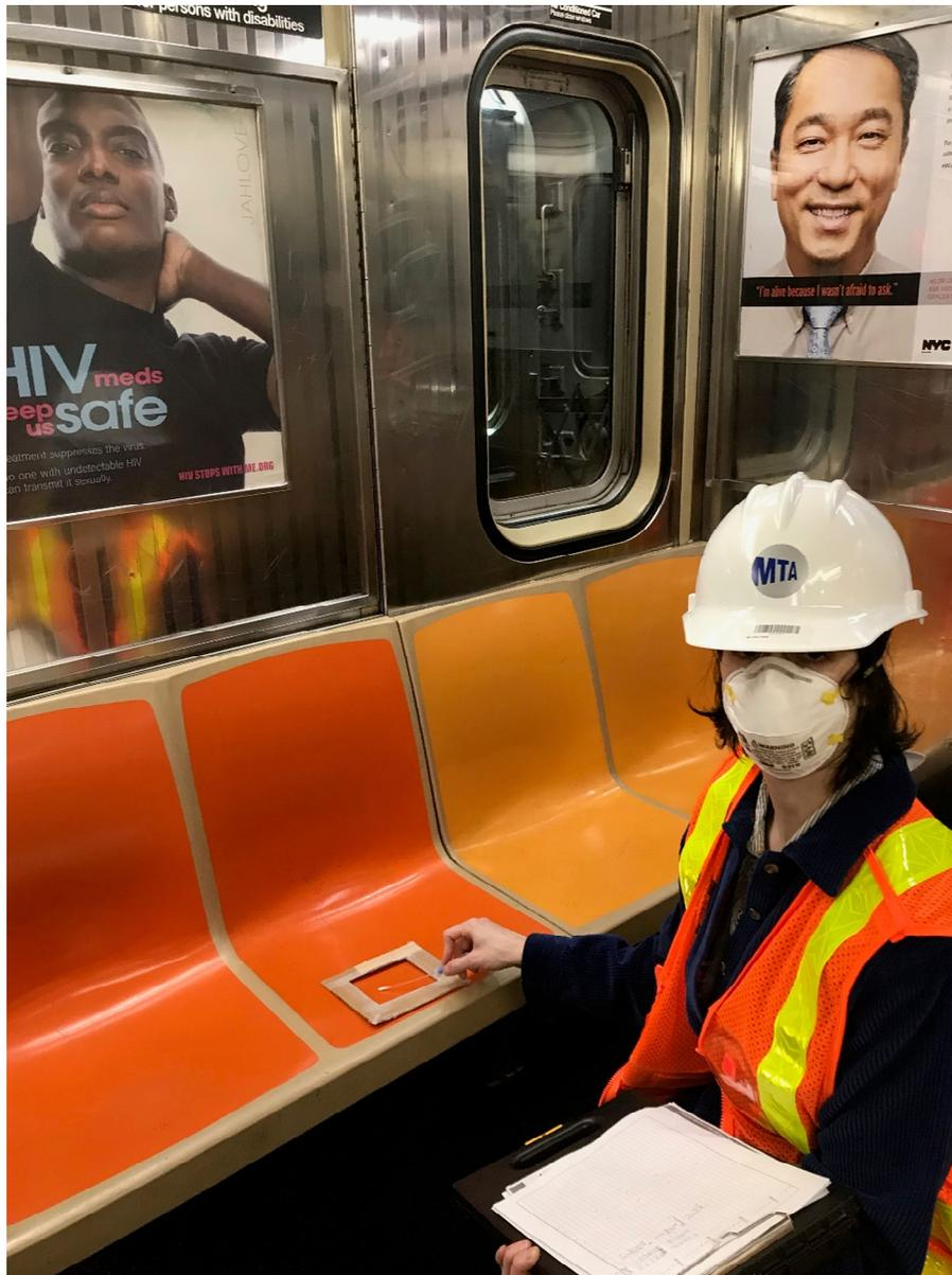
System Safety Specialist Isabel Potter conducts an Adenosine Triphosphate (ATP) sampling event. In this case, ATP testing is being utilized to measure micro-organisms on a surface.
