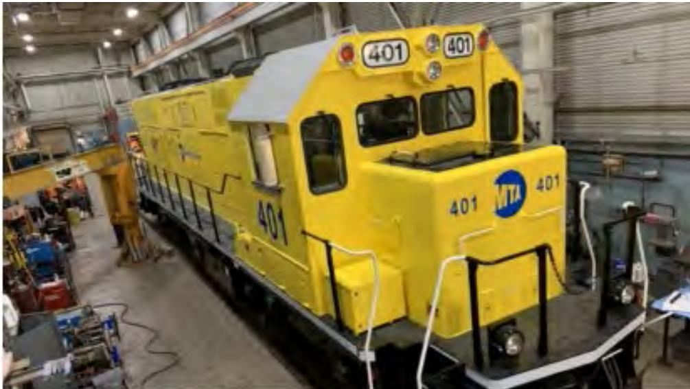
*BL14 Diesel-Electric Switcher unit 401 recently received an overhaul at the Freight & Paint Shop in North White Plains. The project required steel replacement and fabrication, window frame and roof panel replacement, welding, electrical work and painting.*
