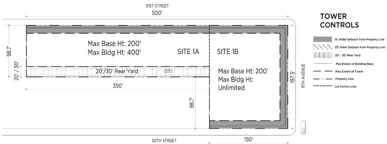
Figure IV-1.1 SITE 1 Ground Floor Controls
