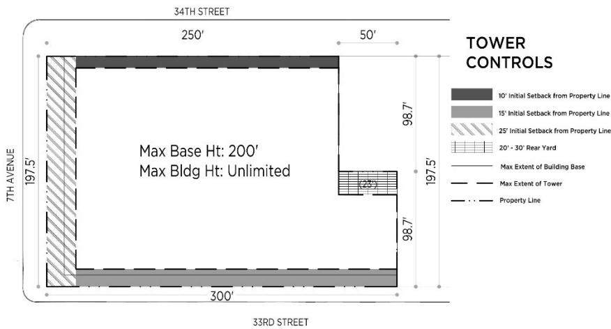
Figure IV-6.2 SITE 6 Tower Controls
