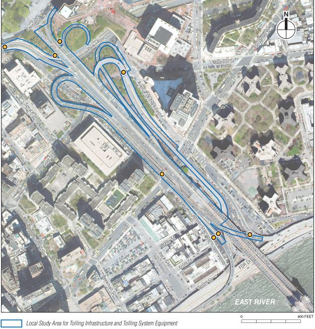
Figure 3-3f. Proposed Locations of Tolling Infrastructure and Tolling System Equipment: Brooklyn Bridge
