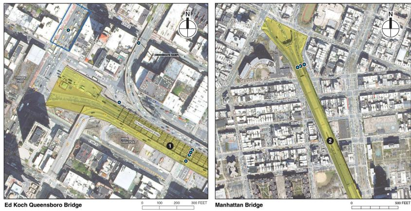
Proposed Location of Tolling Infrastructure and Tolling System Equipment (each circle represents a detection location, which may include one or more new poles or new tolling system equipment mounted on existing infrastructure in that general location)
