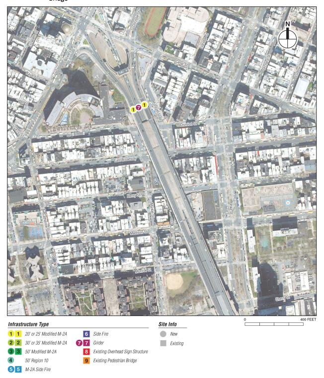
Figure 2-2e. Proposed Locations of Tolling Infrastructure and Tolling System Equipment: Manhattan Bridge
