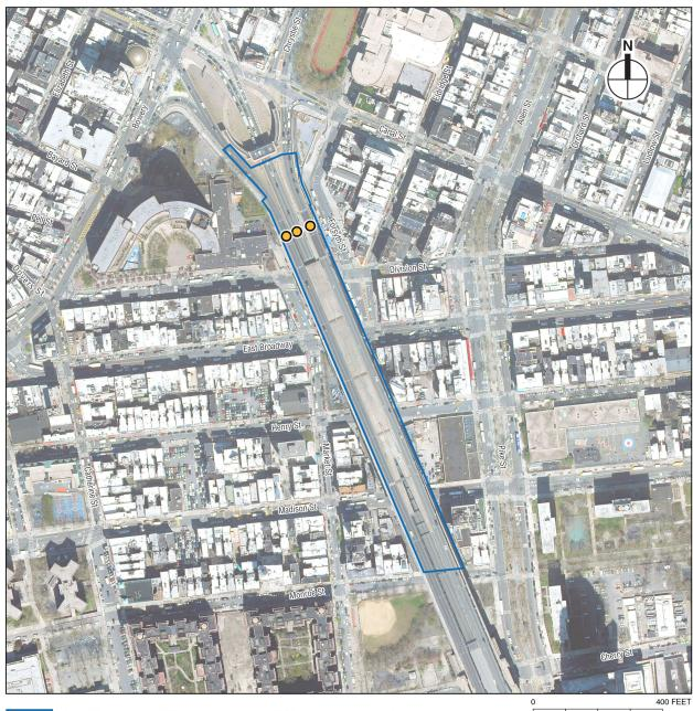
Proposed Location of Tolling Infrastructure and Tolling System Equipment (each circle represents a detection location, which may include one or more new poles or new tolling system equipment mounted on existing infrastructure in that general location)
